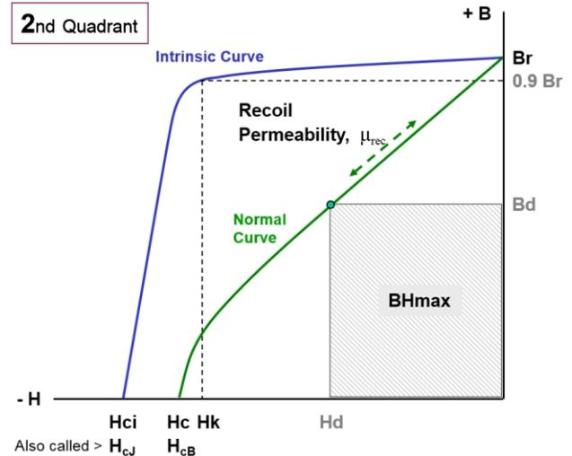
**Figure 2:** Typical 2<sup>nd</sup> quadrant of a hysteresis loop for a permanent magnet material
