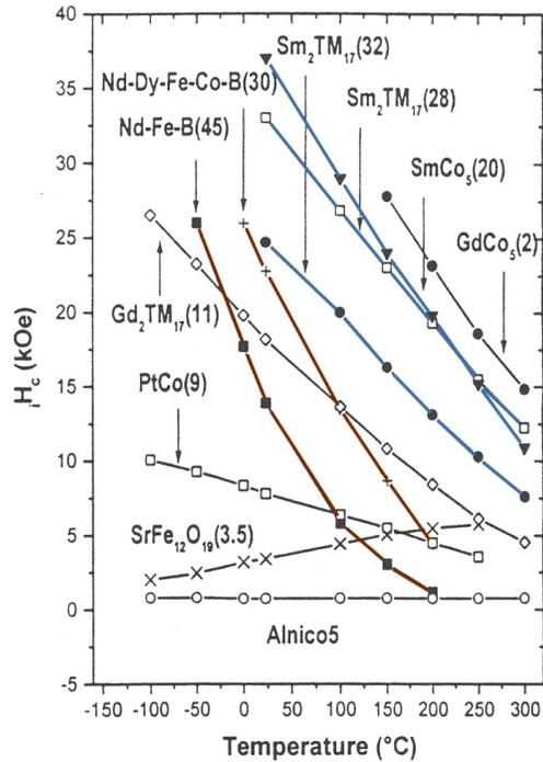
**Resistance to demagnetization in SmCo is also superior to NdFeB, especially at elevated temperatures.**
