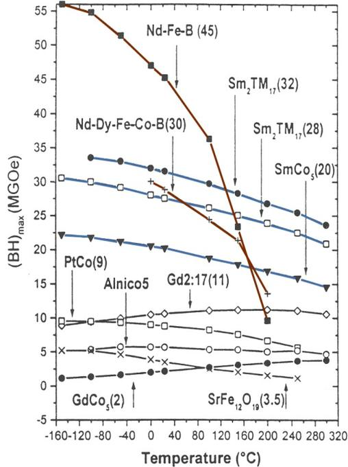
Between  $-138^{\circ}\text{C}$  (135 K) and  $150^{\circ}\text{C}$ , NdFeB outperforms SmCo for flux output. Above  $\sim 150^{\circ}\text{C}$  NdFeB suffers sufficient loss in induction that SmCo is superior.
