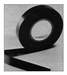
PLASTIFORM® Magnetic Strip 1016 is a flexible bonded magnet which is made using a special process that orients barium ferrite crystals in a polymer binder during manufacture. This orientation process yields a material with excellent magnetic properties.
