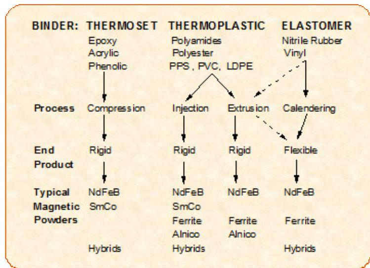
The temperatures used to form bonded magnets are relatively low (less than 340 °C) compared to temperatures used in making the magnetic powders. Therefore, different magnetic powders can be mixed to result in what is called a "hybrid" magnet. Particularly useful hybrids are mixes of ferrite powder with a small amount of rare earth powder, usually neodymium iron
