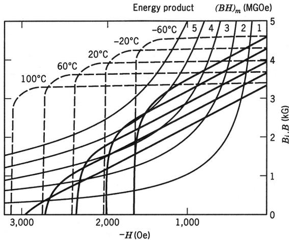
Figure 2. The effect of temperature on the intrinsic and normal curves for ferrite (Ceramic) 5.
