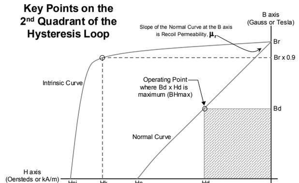
Figure 1. Key Points on the Demagnetization Curve (Second Quadrant of a Hysteresis Loop).
