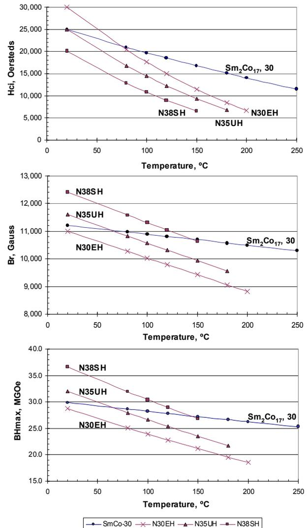
Figure 4. Comparison of SmCo and NdFeB magnetic properties from 20 to 250°C
