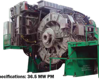
Specifications: 36.5 MW PM Machine for Electric Ship Propulsion
