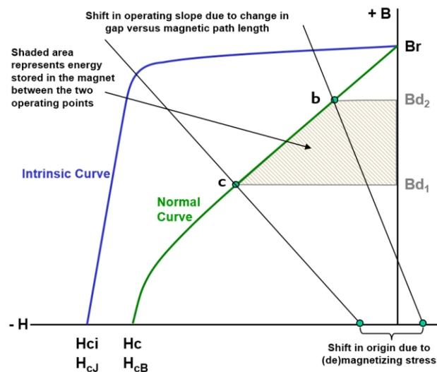
**Figure 3:** 2<sup>nd</sup> quadrant of a hysteresis loop showing change in potential energy as a function of operating points on the normal curve. [4, 5, 6]
