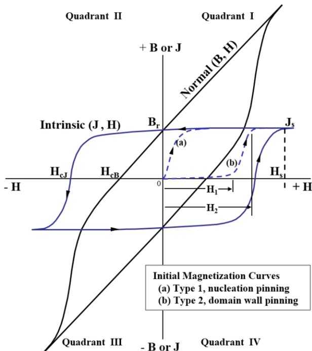
**Figure 1:** Complete normal and intrinsic hysteresis loops with key metrics identified [2]
