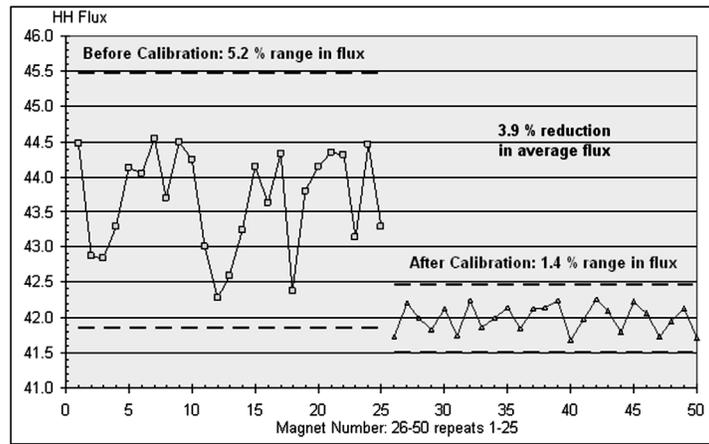
**Figure 8.** Distribution of flux before and after magnetic calibration
