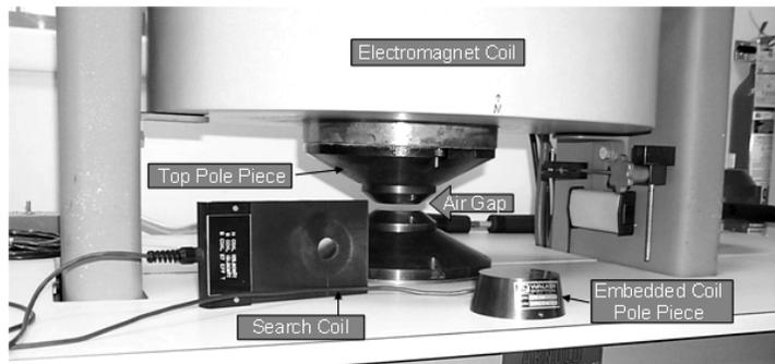
Figure 7. Hysteresisgraph showing search coil, pole caps and electromagnet. Embedded pole cap can be substituted for standard pole cap.
