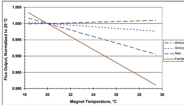
Figure 6 chart of normalized flux change as function of temperature
