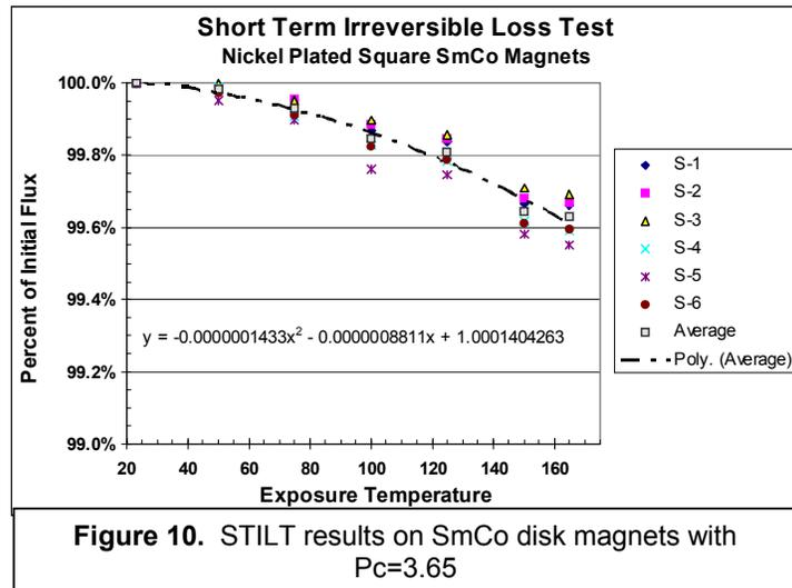
is suspicion of chemical reaction or corrosion occurring, it may be desirable to re-saturate and re-measure the magnets. The amount by which they fail to return to 100% of initial output represents irreversible loss, most likely from structural damage.
