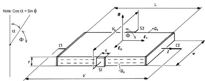
Figure 2. Schematic of a Hall chip<sup>(7)</sup>
