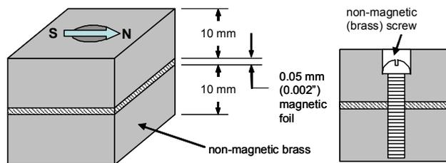
Figure 3. Hall Probe Element Locator
