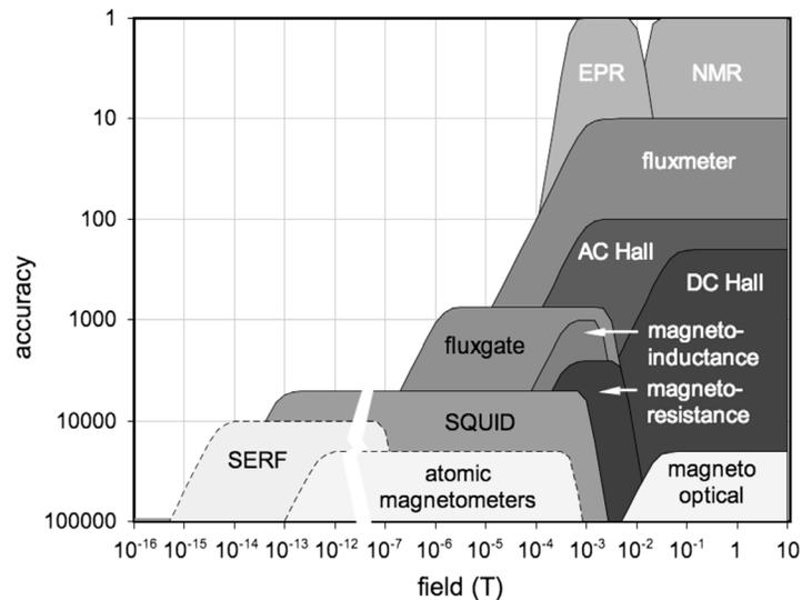
**Figure 1.** Accuracy and sensitivity of magnetic field measuring devices
