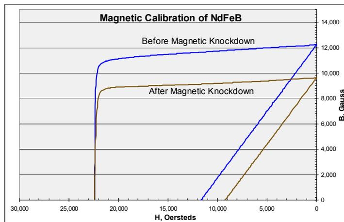
**Figure 9.** Hysteresisgraph curves showing drop in  $B_r$  with magnetic knockdown while  $H_{cJ}$  remains unchanged
