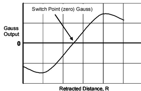
Figure 4. Finding Hall chip neutral plane by change in polarity of the field
