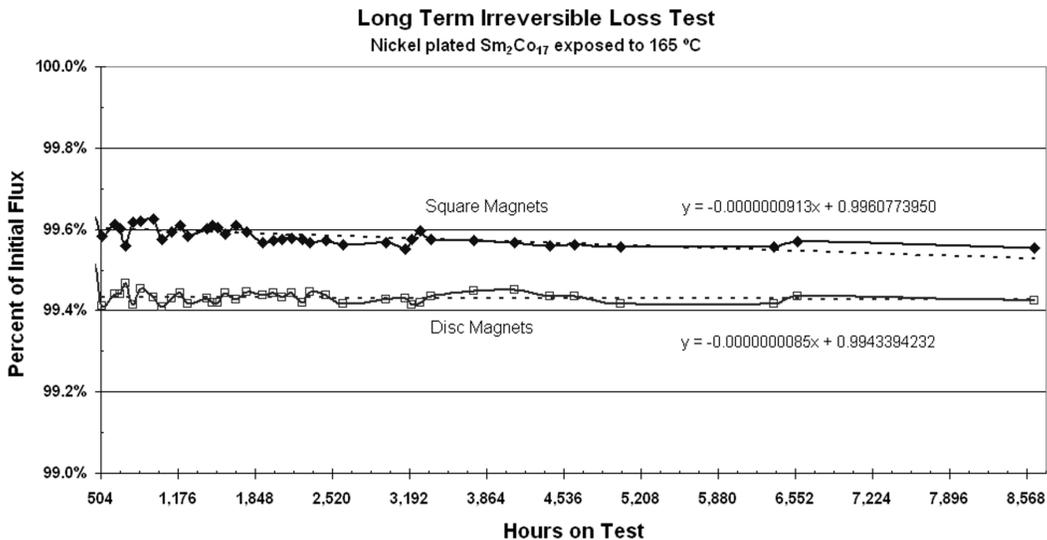
**Figure 11.** LTILT of nickel plated SmCo exposed to 165 °C for several thousand hours
