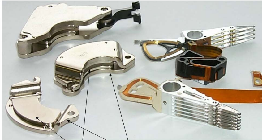
Nickel plated magnets and steel return paths.
