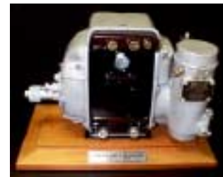
Figure 7. Delco Self-starter-generator unit - 1912
