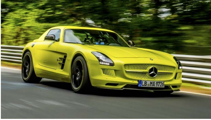
Mercedes-Benz SLS AMG Electric Drive: 740-hp super-sports car with one electric motor per wheel
