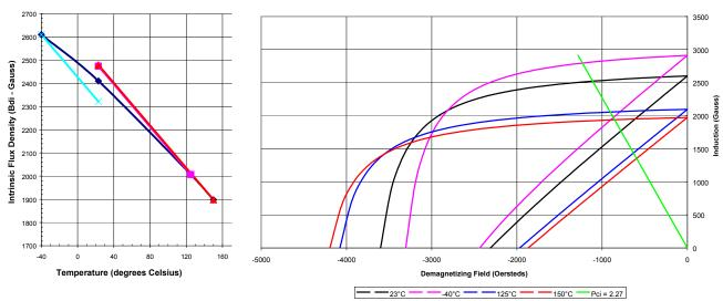
Anisotropic 2060 Typical Demagnetization Curve
