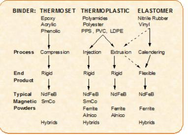
The temperatures used to form bonded magnets are relatively low (less than 340 °C) compared to temperatures used in making the magnetic powders. Therefore, different magnetic powders can be mixed to result in what is called a "hybrid" magnet. Particularly useful hybrids are mixes of ferrite powder with a small amount of rare earth powder, usually neodymium iron
