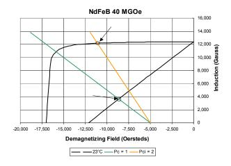
Using the intersection of the intrinsic (magnetization) curve and the Pci slope one obtains the magnetization of the magnet under the reverse applied field. Adding the Bdi and Hd values results in Bd under the influence of the reverse field (Bd = Bdi + Hd; remember Hd is a negative value in the second quadrant).
