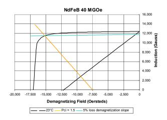
If the Pci is reduced to 1.5 (Pc = 0.5, Pci = 1.5), then the amount of reverse field that may be applied without demagnetization is less. This
