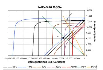
When there is no reverse applied field, the Pc and Pci lines intersect the normal and the intrinsic curves respectively and have the same Hd value. This condition is only true when there is no reverse applied field.
