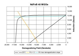
It should be noted that for a Pci = 2 that the reverse applied field required to demagnetize to this extent is ~9,300 Oersteds (740 kA/m). The magnet will operate on this reduced (stabilized) intrinsic magnetization curve as long as the demagnetizing influence for a Pci = 2 does not exceed the stabilizing value of 9,300 Oersteds reverse applied field.
