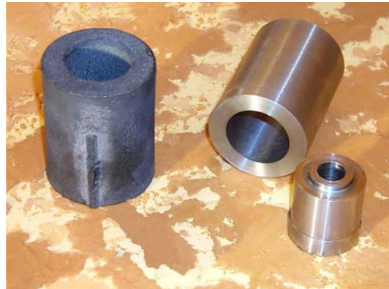
Cast Arnokrome III is machinable with standard metal-working tools.
