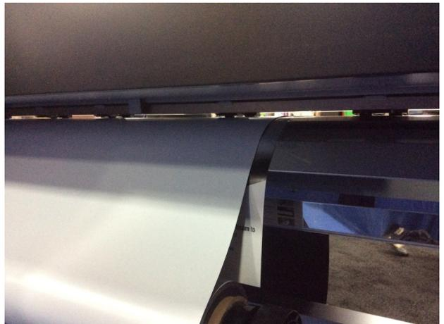
Wide Format Printers: Some wide format inks need heat to dry quickly. Because the heavy magnetic base acts as a heat sink, the tendency may be to increase the heat setting to dry the ink. This may cause the magnetic base to soften, and the heavy weight of the stock may cause it to stretch. It is best just to use lower heat and allow the ink more time to air dry.
