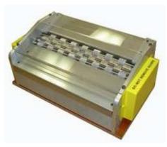
**Industrial Magnetizers:** Flexmag manufactures several industrial units in widths from 13" up to 26". These motorized magnetizers have a variable speed control that runs up to 145 feet per minute, and they will permanently magnetize substrates up to .060" thick - both standard and high energy.
