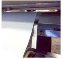
heat sink, the tendency may be to increase the heat setting to dry the ink. This may cause the magnetic base to soften, and the heavy weight of the stock may cause it to stretch. It is best just to use lower heat and allow the ink to air dry. For latex printers, we recommend either our Ultra-Mag Non-Top Coated Vinyl or Flexcoat-EZ.
