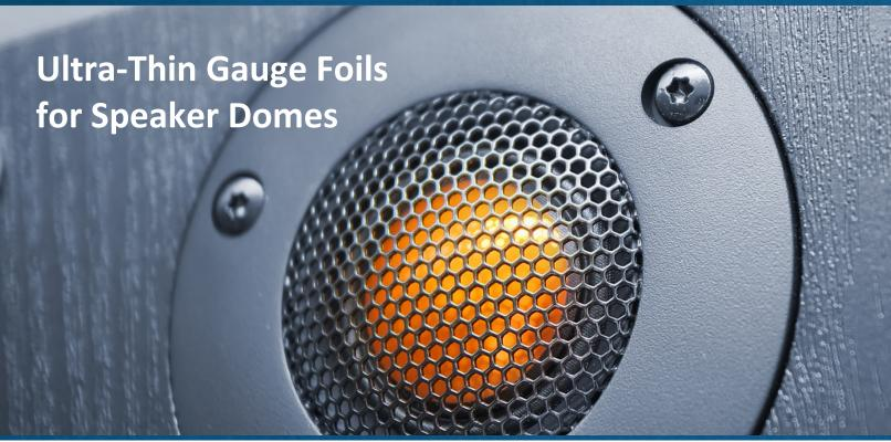
Today's consumers demand exceptional sound quality from their speakers. One of the main components involved in the delivery of crisp, clear sound is the speaker dome. It is important that the dome be made of a clean ultra-thin metallic foil to allow efficient transfer of the electrical signal into sound waves over a wide range of frequencies. Also, in order to prevent failures in the speaker's operation, the foils must have a defect-free surface finish.
