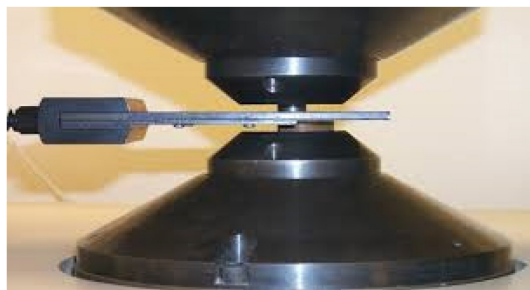
Figure 7. A magnet sample (in the center) between the pole pieces in a hysteresisgraph. The sample is surrounded with a flat coil set.
